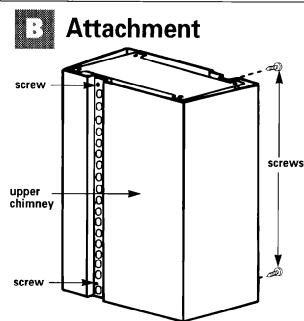
Remove the four screws on the upper chimney and disassemble chimney pieces from support frame.
